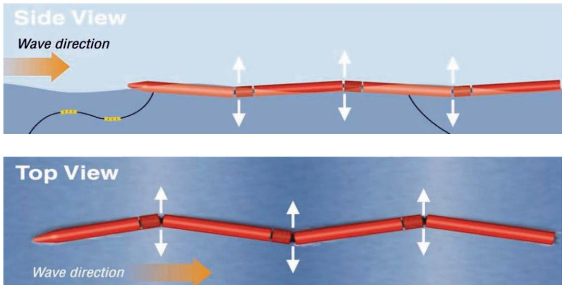
The hydraulic rams drive pressurised fluid into power smoothing, high pressure accumulators which then direct the fluid through variable displacement motors and back to low pressure fluid reservoirs. The variable displacement motor is directly linked to an asynchronous generator producing a 3-phase voltage.
