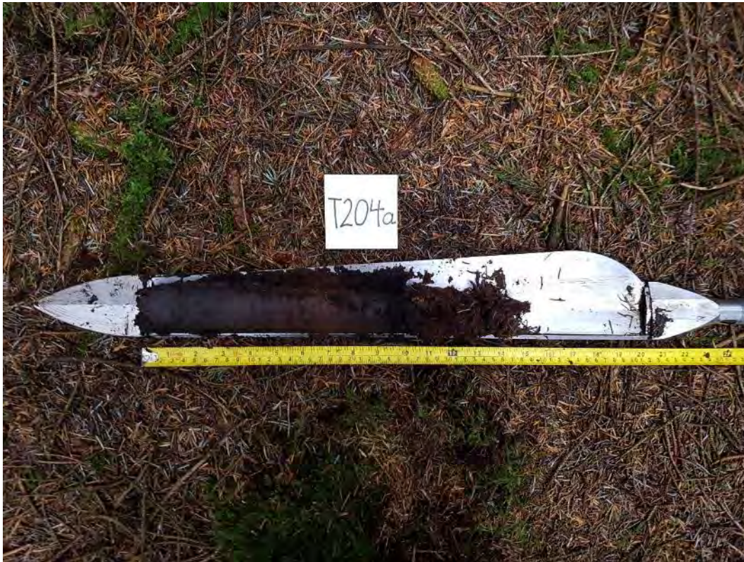
Core Sample T204a – Turbine 1
