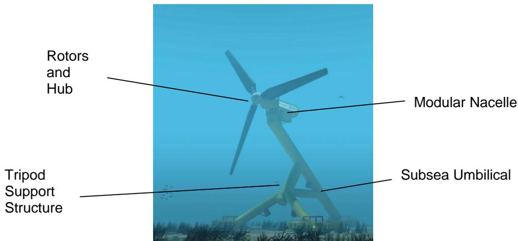
Figure 2: A schematic of the 300kW device
