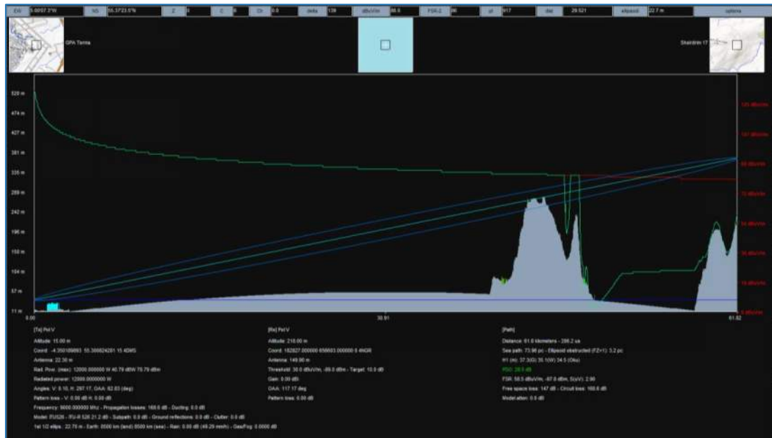
Figure 9: Path loss profile between GPA Terma PSR and tip of turbine 17
