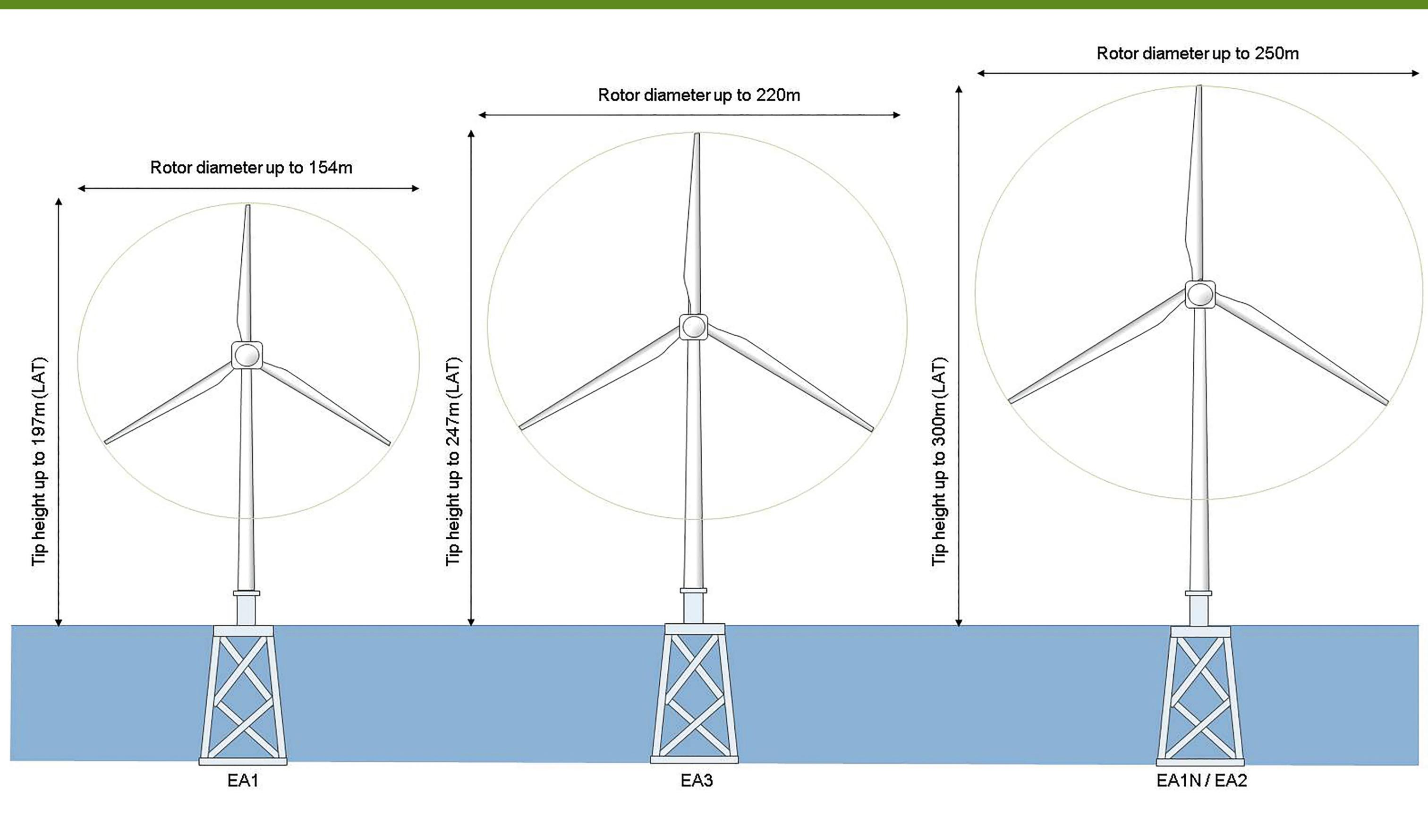
The technologies used in offshore wind turbines are constantly evolving and the industry is moving towards larger more powerful wind turbines. For these projects up to 19MW wind turbines are being considered. The benefits of installing larger machines are:
