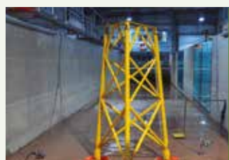
A scale model of East Anglia ONE jackets undergoing tests at HR Wallingford
