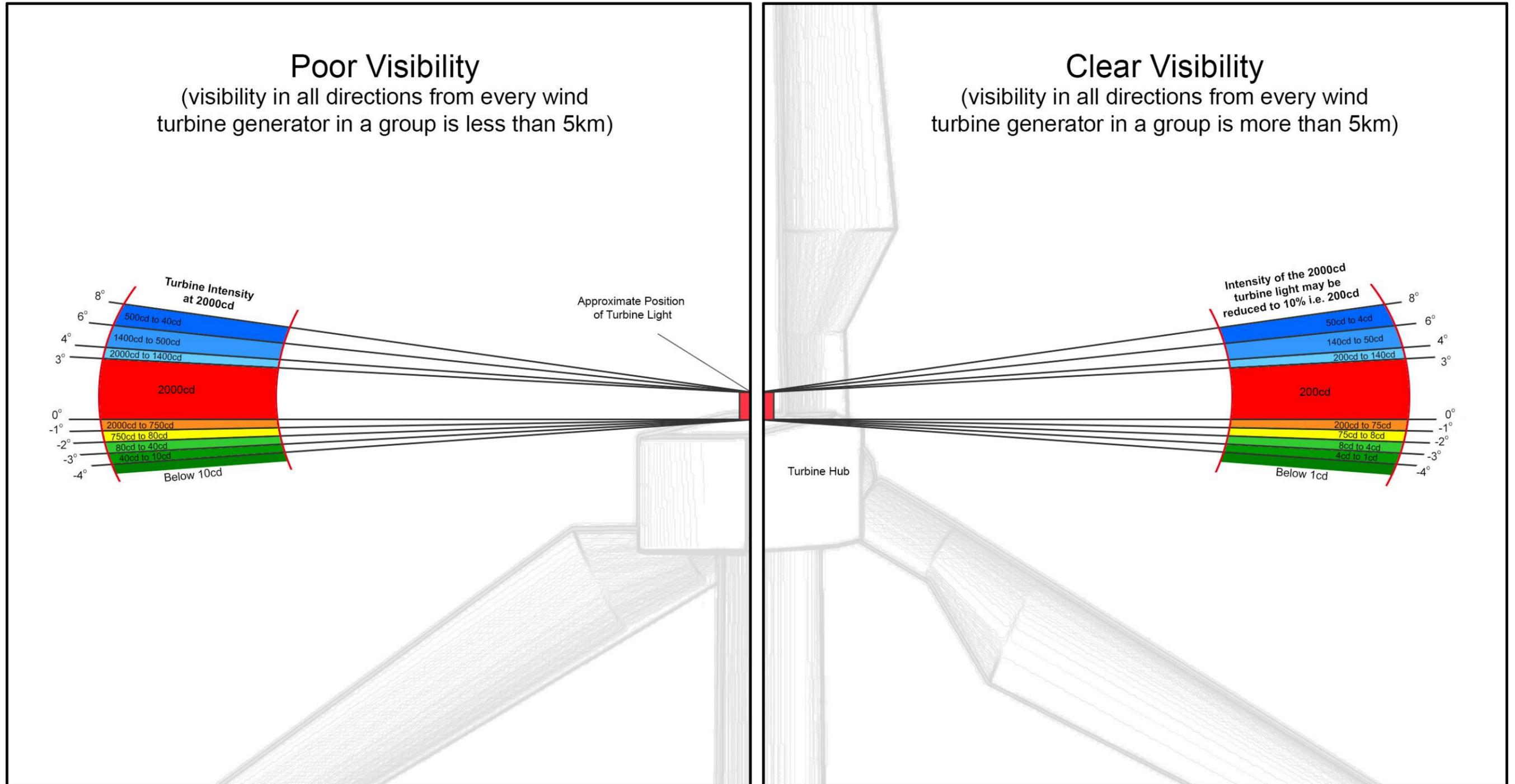
Plate TA 6.2.2 Diagrammatic interpretation of minimum requirements of ICAO/CAP393 (LuxSolar Medium Intensity Obstruction Light)
