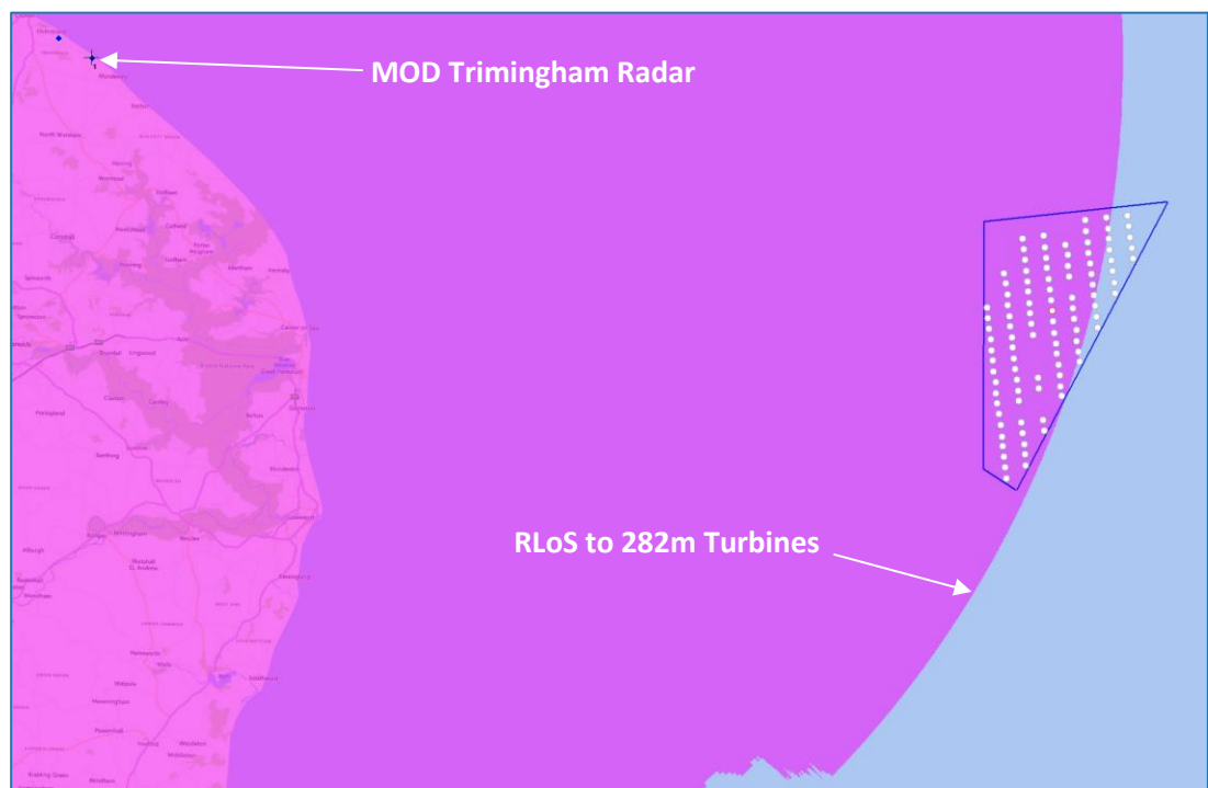
Figure 4: Trimingham Radar RLoS to 282m Tip Height Turbines
