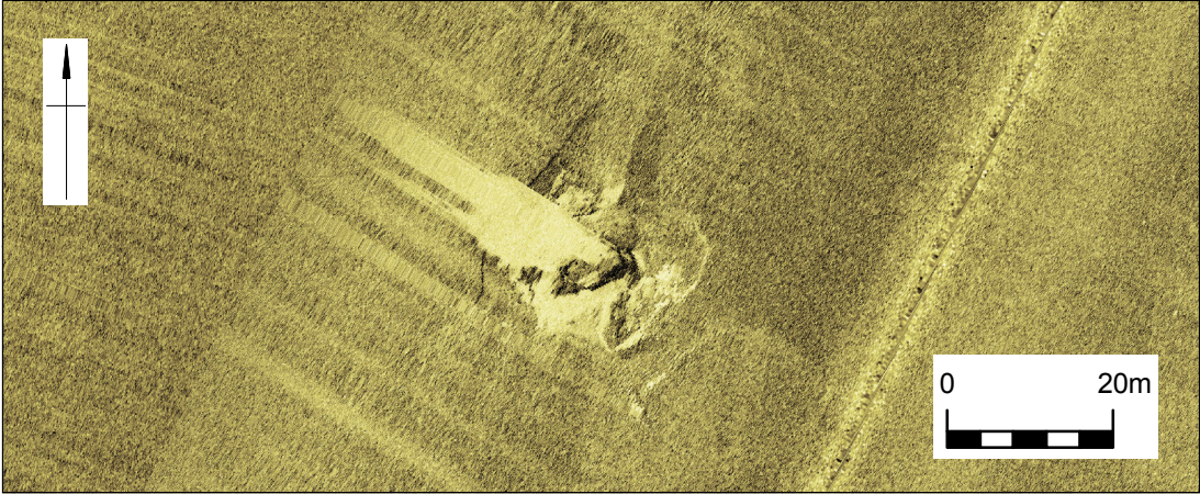
Sidescan sonar image of 700605 , 10.0 m x 6.9 m x 4.9 m
