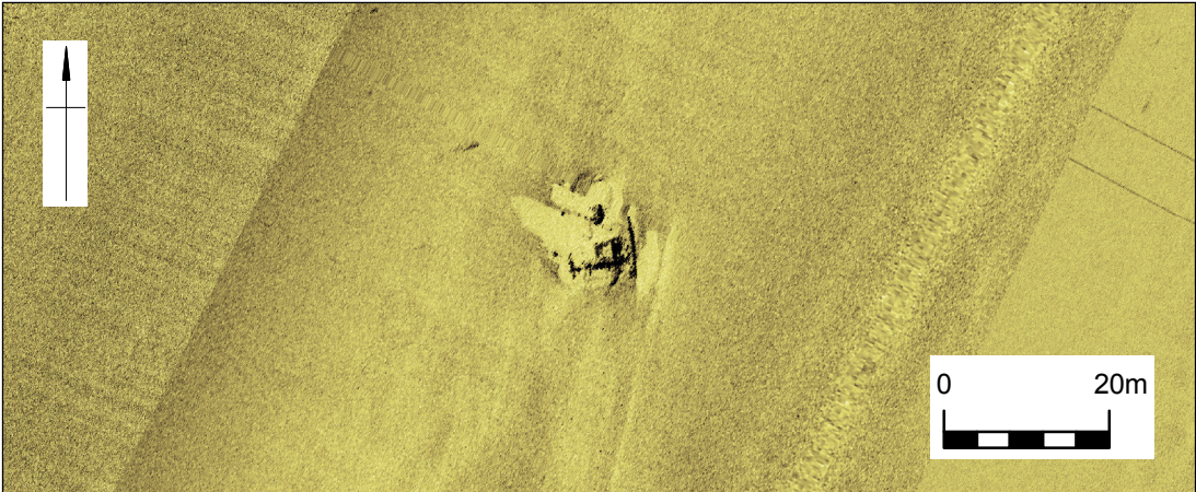
Sidescan sonar image of 700590 , 13.3 m x 13.1 m x 1.6 m
