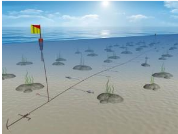
Diagram A13.1.10 Longlines (source: Seafish, 2015)
