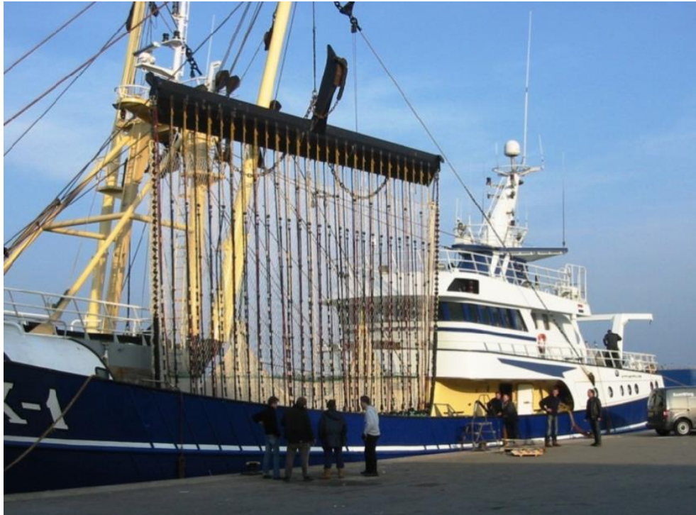
Plate A13.1.9 Dutch fishing vessel with a pulse wing trawl (Eayrs & Suuronen, 2013)
