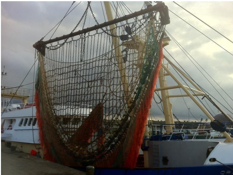
Plate A13.1.8 Traditional beam trawl net with tickler chains and chain mat (BMM, 2012)
