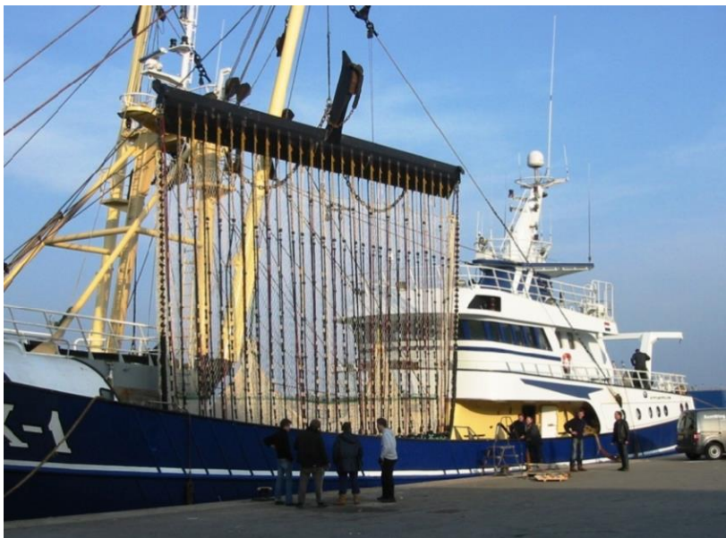
Plate A13.1.8 A Dutch fishing vessel with a pulse wing trawl (Eayrs & Suuronen, 2013)
