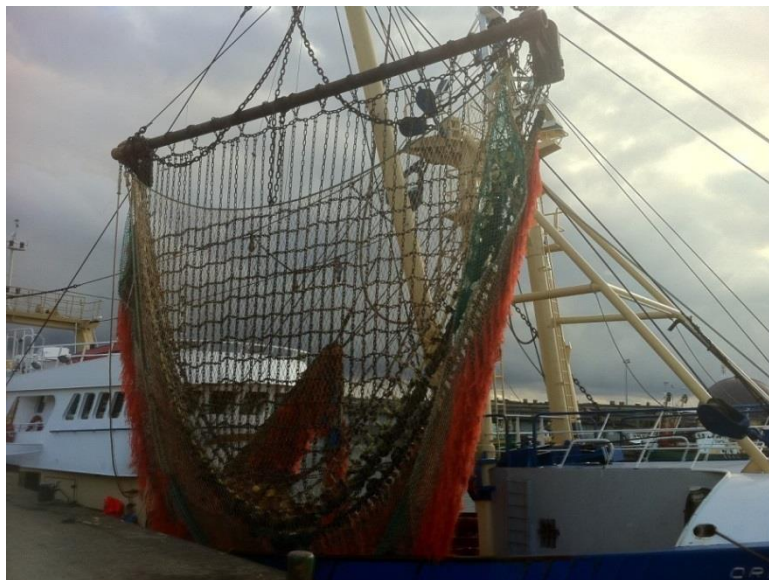
Plate A13.1.7 A traditional beam trawl net with tickler chains and chain mat (BMM, 2012)
