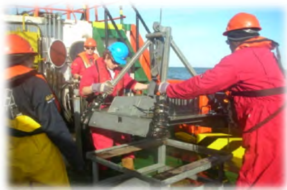
Plate 2. Retrieving the 0.1m 2 mini-Hamon grab on board the MV Ivero during the EAOW zonal survey. © www.seasurvey.co.uk
